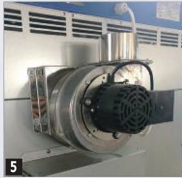
5 Air outlet extractor
