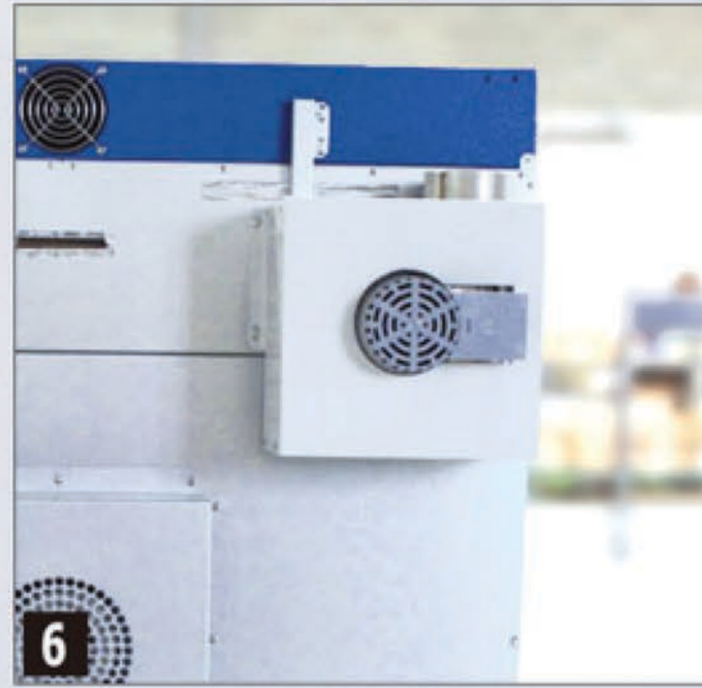
6 Air cooling extractor
