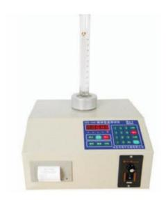
Tapped Density Analyzer or Tapped Density Meter . AS-100 Tapped Density Tester is a density measurement equipment used to measure the tapped density of powders, as well as granulated or flaked materials by standardized and repeatable procedures
