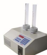
Tapped Density Tester AS-100
